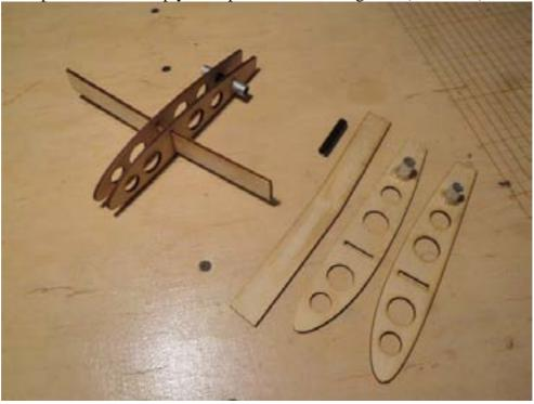
16. Glue the plywood profiles to the sides of the central, left and right wings. Make sure that the holes in the plywood profiles for the spar joiners properly fit to the joiner boxes.
