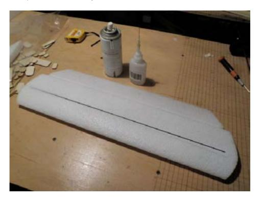
19. Glue two carbon flats in to the rudders. Cut out a square hole to insert the rudder's servo and strenghten it with a plastic element. Glue the rudder's control arms.
