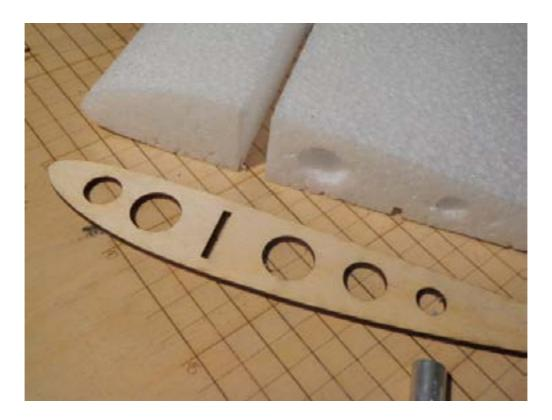
15. Glue alu pilot sleeves into plywood profiles of the wing ends (rear holes) with resin.
